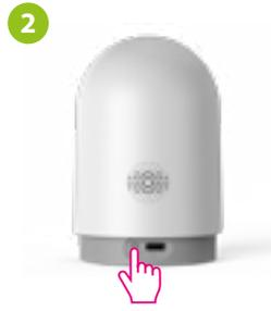
Make sure the camera is powered on. Then press and hold the button on the back of the camera for approximately 5 seconds, until the beep. The blue LED on the front of the unit will then start flashing. The pairing mode is enabled.
