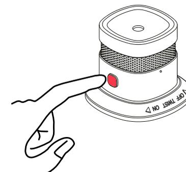
To test or to mute the alarm, press and hold the Test / Mute Button for 3 seconds.
