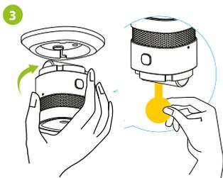
Remove the battery insulating strip to turn on the detector and rotate the sensor clockwise into the bracket.
