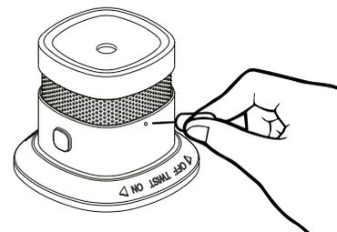
To set the device into pairing mode, press and hold the pairing button for 3 seconds.
