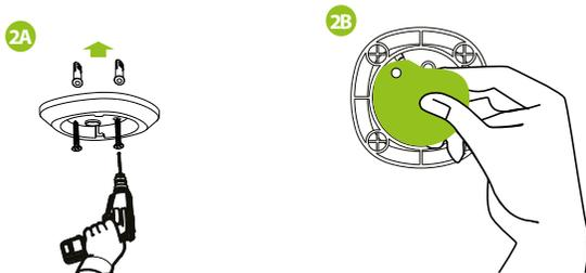
Install the bracket using the screws or the provided doublesided tape.
