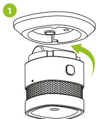
Rotate the sensor anticlockwise to separate it from the bracket.
