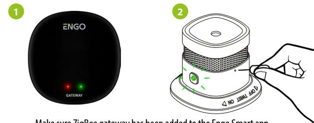
Make sure ZigBee gateway has been added to the Engo Smart app. Press and hold the pairing button with the attached pin for about 3 seconds until the green LED starts flashing. The sensor will enter pairing mode.
