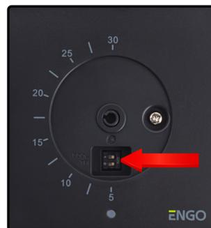
Additional functions of the thermostats can be switched on or off by switches, which are located on the front cover, under the knob. Refer to the table below to understand what these features are:
