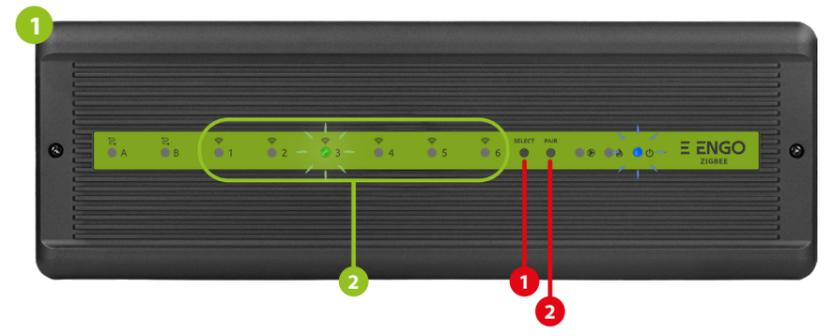
In order to correctly link thermostat with the control box, first select the zone in the control box with the SELECT button (1) (zone which you want to link with thermostat). The LED (2) will flash 3 times for the selected zone. Confirm your selection by clicking PAIR button (2). The LED (2) will flash green with the previously selected zone - binding process has started, it is active for 10 minutes and during this time you can link thermostat with the selected zone.
