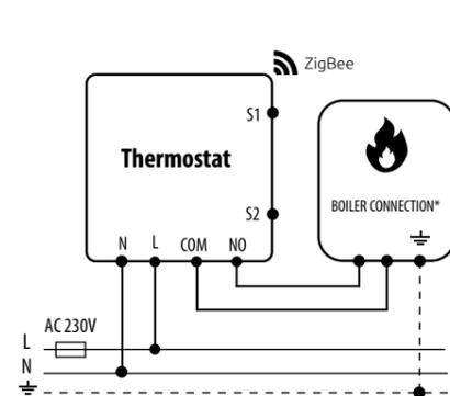
b) Connection diagram to pump / actuator:
