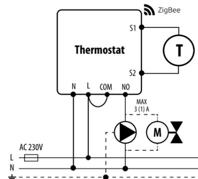
c) Connection diagram to the control box:
