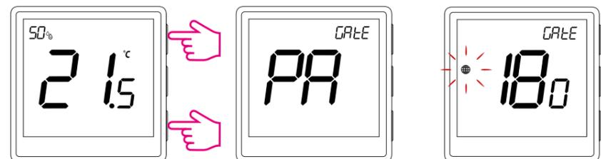
Make sure ZigBee Gateway has been added to the Engo Smart app. Press and hold the ▲ and ▼ buttons on the thermostat until the display shows „PA“. Then release the keys. The pairing mode will be started up.
