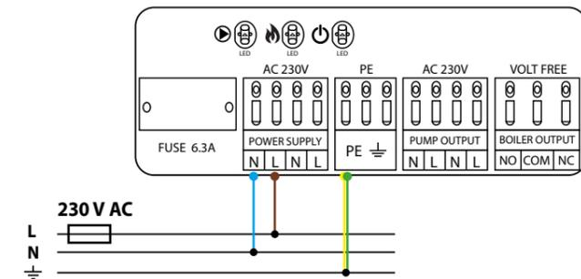
Power supply for wiring centre is 230 V ~ 50Hz.
