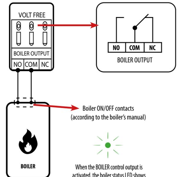
When the BOILER control output is activated, the boiler status LED shows a constant green light.
