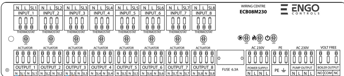
**Please note:** Depends on the thermostat heating state - 230 V AC may appear on the actuators output.
