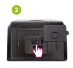
Make sure the camera is powered on. Then press and hold the button on the back of the camera for approximately 5 seconds, until the beep. The blue LED on the front of the unit will then start flashing. The pairing mode is enabled.
