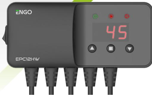
The controller turns on when the boiler temperature exceeds the user-set central heating pump activation temperature. The DHW pump works on the basis of a temperature difference. The DHW pump is switched on when the boiler temperature exceeds the tank temperature by the hysteresis set by the user. The hot water pump works until the boiler and tank temperatures equalize or the set tank temperature is reached.
