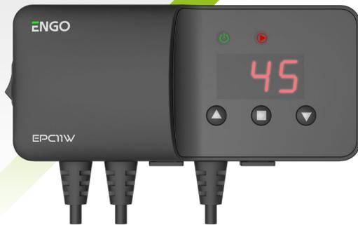
It is designed to control the water pump in the central heating and hot water circulation. It also works as a safety thermostat. It has the ability to turn on and off the pump. The pump will start after exceeding the temperature set by the user „C”, and will turn off after exceeding the set off temperature „U”.
