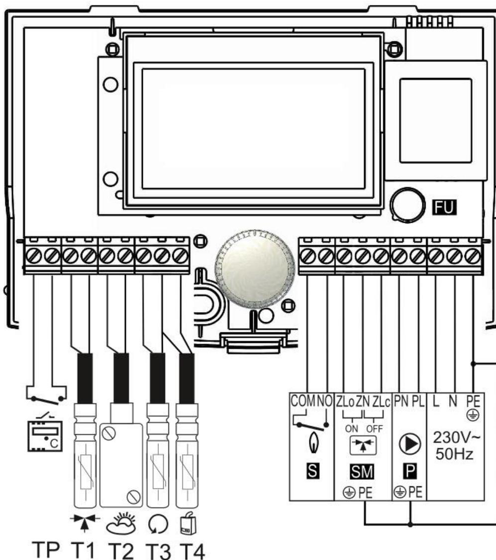
TP – room thermostat (No-Nc), T1 – temperature sensor mixer heating circuit type CT10, T2 – external temperature sensor type CT6-P, T3 – return temperature sensor type CT10, T4 – heat source temperature sensor type CT10, L N PE – power supply 230V~, 50Hz, P – CH pump, SM – mixer actuator, S – contact to operate the heating source type ON-OFF, FU – time-delay subminiature fuse.
