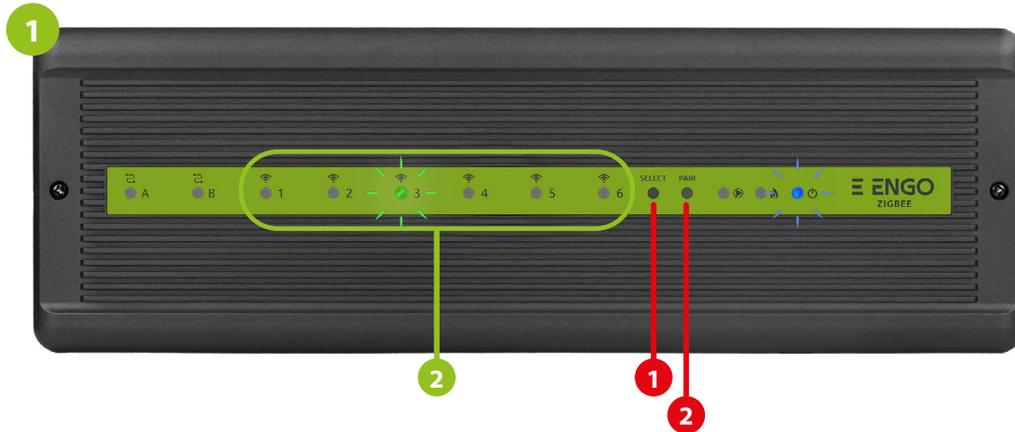
In order to correctly link thermostat with the control box, first select the zone in the control box with the SELECT button (1) (zone which you want to link with thermostat). The LED (2) will flash 3 times for the selected zone. Confirm your selection by clicking PAIR button (2). The LED (2) will flash green with the previously selected zone - binding process has started, it is active for 10 minutes and during this time you can link thermostat with the selected zone.
