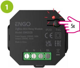
To properly bind thermostat with the module first click quickly the button on the device 5 times. The LED diode will start flashing slowly on red, which means the device will enable binding mode.
