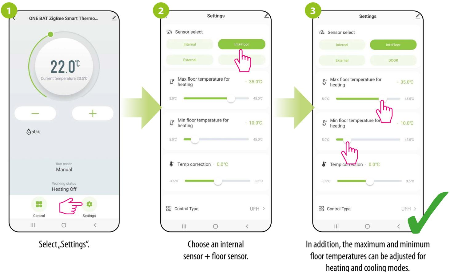
**External temperature sensor (as an air sensor)** - if an external sensor is connected to the S1/S2 terminals and selected external sensor, the thermostat will display the temperature from this sensor ignoring the internal sensor. The external temperature sensor can be used in case where the thermostat need to be in other place than controlled room.
