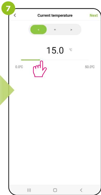
Use the slider to set the value of room temperature, below which you will receive a notification of low room temperature.
