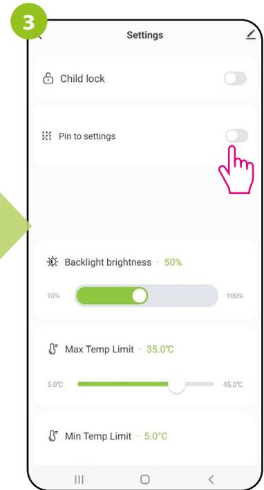
If the „Pin to settings“ is enabled then user of the thermostat each time will need to enter a PIN to enter the installer settings.
