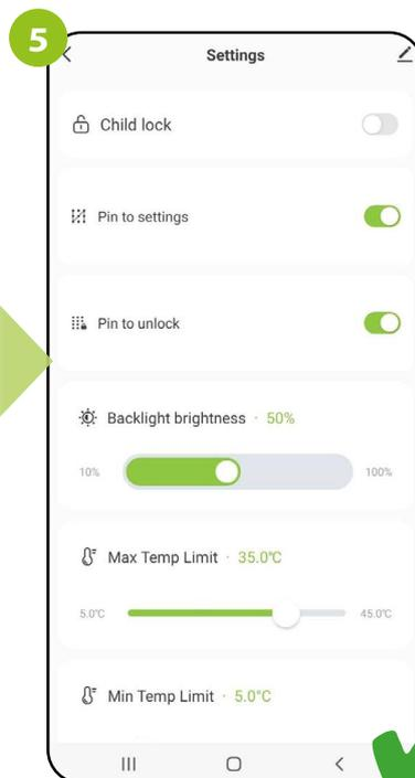
If the „Pin to unlock“ is enabled, the user will always need to enter pin code to unlock thermostat buttons.
