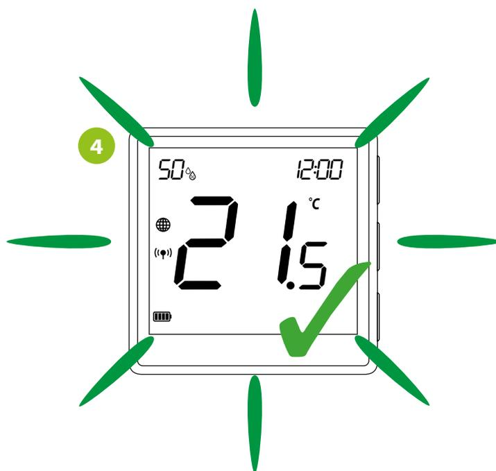
When the slider is moved (see previous step), the thermostat display automatically changes its brightness.
