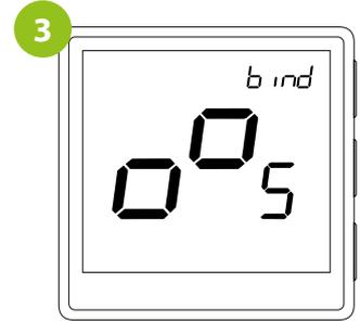
Release the keys, binding function (process of linking thermostat) is active.
