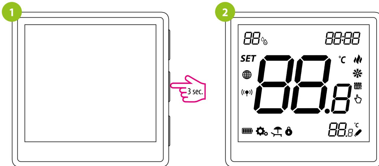
To power on the thermostat hold ✓ button for 3 seconds...
