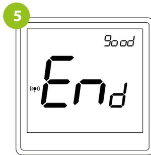
After successful binding operation „End” message will be displayed. The LED on the module will stop flashing.
