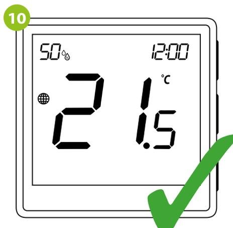
On the thermostat screen appeared an icon globe indicating that it has been added to the ZigBee network.
