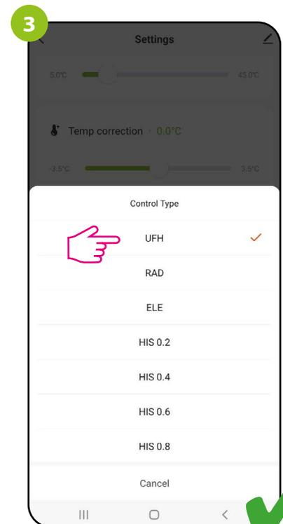
Then select the type of control heating system. Depending on your choice, the thermostat will better adjust its work.
