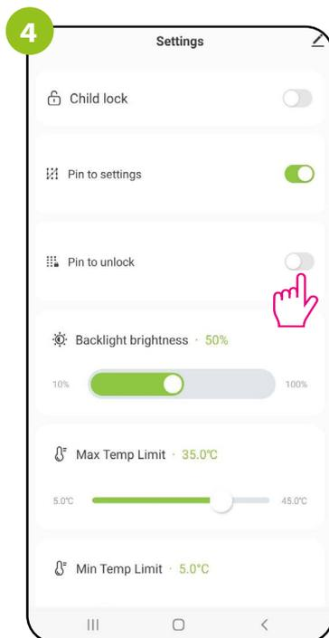
If the „Pin to settings“ is enabled, a new parameter appears - „Pin to unlock“ (thermostat keys).
