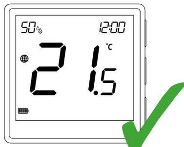
On the screen of the thermostat appears an globe icon indicating that it has been added successfully to the ZigBee network.
