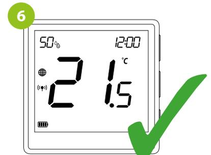
Both devices have been successfully linked. Thermostat displays the main screen, icon (⦿) appeared on the screen indicating connection with the receiver.
