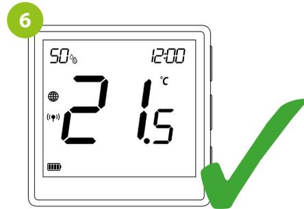
Both devices have been successfully linked. Thermostat displays the main screen, icon (☉) appeared on the screen indicating connection with the receiver.
