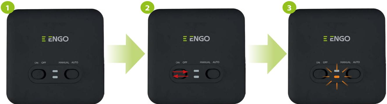
If you want to re-pair the devices with each other, make sure that the receiver is disconnected from the power supply and the switches on it are in the ON and AUTO positions. Then connect the receiver to the power supply.
