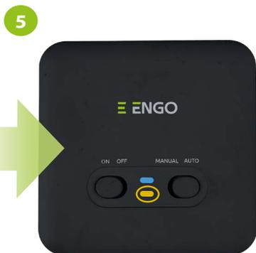
5 Check that the orange LED on the receiver is on. If so, it means that the communication between the devices is correct.
