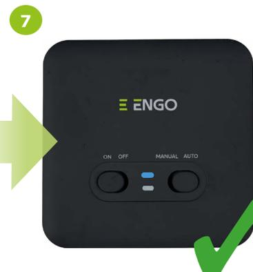
7 ...and the orange LED on the receiver should go out.
