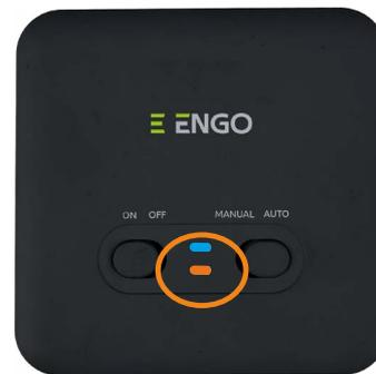
When the orange diode on the receiver lights up continuously, the devices have been paired on a new frequency.
