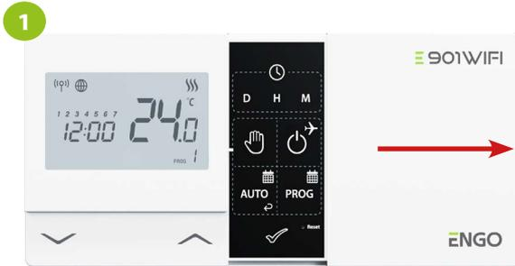
Remove the thermostat cover as shown in the picture. If there are batteries inside, remove them.
