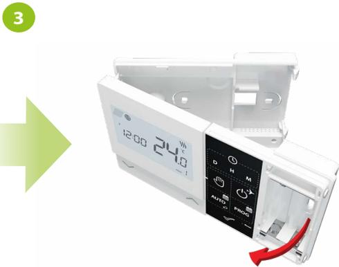
Separate the front part from the back part in the direction shown above.
