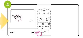
Using or buttons set the hour for the time period and then confirm by button.
