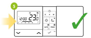
Then the "hand" symbol will disappear from the display and the thermostat will return to the automatic mode.
