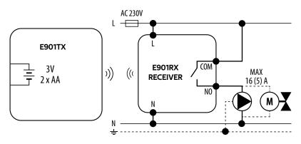
c) Connection diagram to the control box
