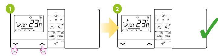
Press and hold  $\wedge$  and  $\checkmark$  buttons for 3 seconds.
