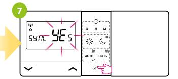
Using or buttons choose YES and start the pairing process on a new frequency by pressing the button.
