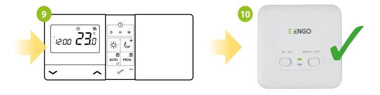
Set the temperature setpoint a few degrees lower than the room temperature by repeating steps 1 to 5. Wait a few seconds. The flames icon should stop animating...
