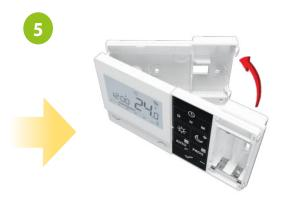
Using the hinges, fold the back and front covers by moving as shown in the picture above.
