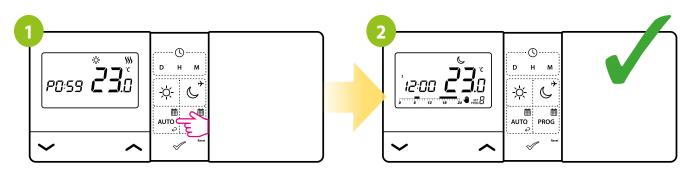
To cancel the function, press any button to turn on backlight and then press 2 times AUTO button.
