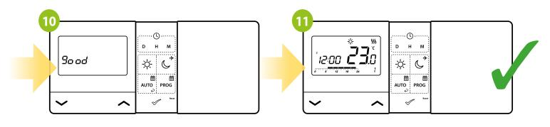
The thermostat will display the message "good", which means that the devices are successfully paired with each other.
