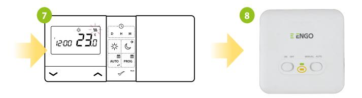
The flame icon will start to animate, which means that the thermostat is sending a signal to heat.
