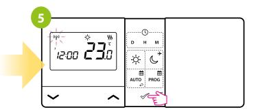
The thermostat started sending a heating signal when the screen went blank, which was signaled by the antenna symbol.
