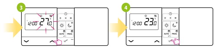
Using  $\sim$  or  $\sim$  buttons set new comfort temperature value.
